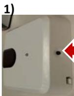
Press and hold for 10seconds and release the back button on the device.
